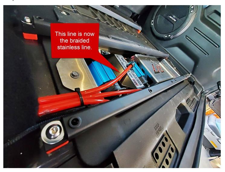
Now is the time to wire your compressor if that has not been done. Please refer to the wiring instructions that came with your compressor. The switch harness should be routed with the air lines during this step.
