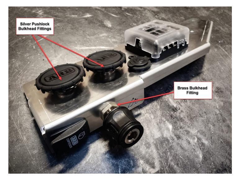
The two silver pushlock bulkhead fittings are used for the ARB filters. When you install the filters into the silver pushlock fittings, it is not necessary to use thread sealing tape.
